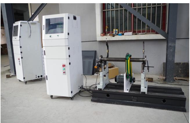
YYQ-160 horizontal hard support balancing machine
