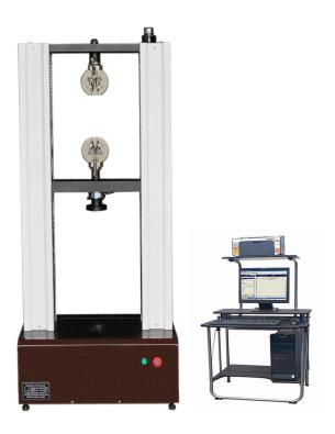
HDW series computer electronic universal testing machines are designed and manufactured according to ASTM, ISO, DIN, GB and other international standards.
