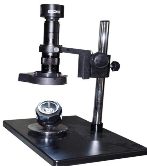
Fig. 2 Wear spot measuring microscope
