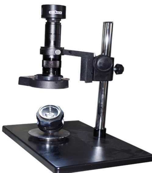
Fig. 2 Wear spot measuring microscope
